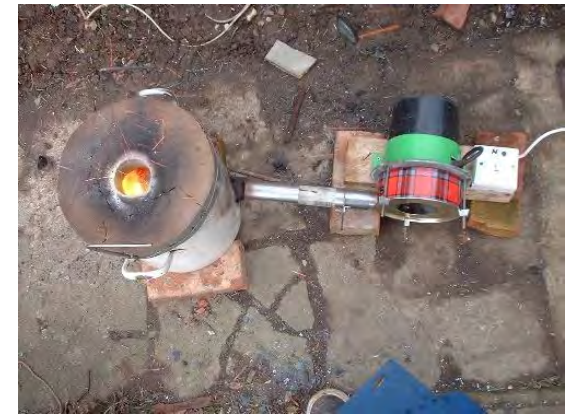
Colin Pecks paraffin burner which uses a dryer motor and cookie tin in the construction.
